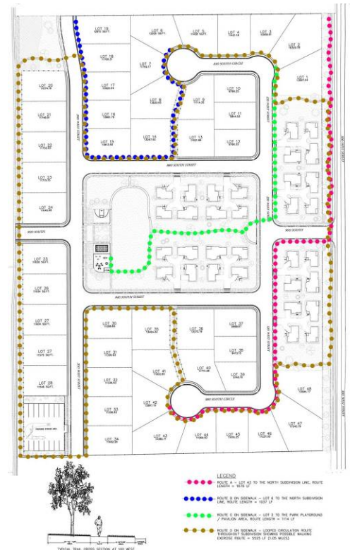
Trail Routes Plan showing trail and sidewalk connections through the development and a typical trail cross section
